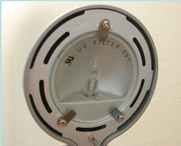
A Tungsten-Halogen lamp with a filter to remove UV light.
